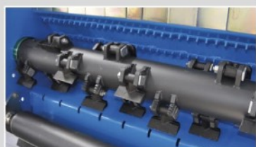
Controcoltelli dentati e supporto mazze dentato Notched counter-knives and notched hammer holder
