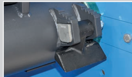
Mazza pesante e perno Ø25 mm trattato Heavy hammer with hardened axle of ø 25 mm.
