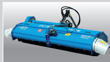
Coclee coassiali con spirali opposte per la pacciamatura da ambo i lati. Coaxial spirals with opposite helixes for mulched stubble delivery on both sides.
