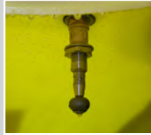
Getto rotante lava cisterna Internal nozzle for tank washing Inyector interno lava tanque
