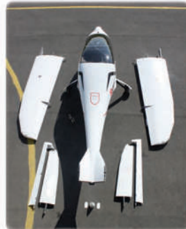
REMOVABLE WINGS & TAIL FOR TRANSPORT
