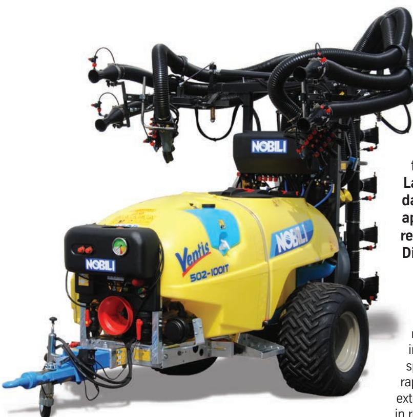
The handling of the structure is facilitated by a system with three hydraulic cylinders (lifting, right and left opening) and two electric actuators that regulate the inclination of external cannons.
