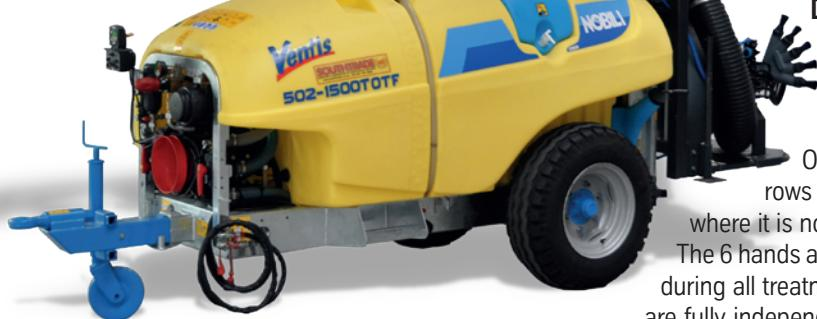
Simple and compact structure, mechanically adjustable in width and hydraulically adjustable in height and for arms opening up to 3,5 meters.
